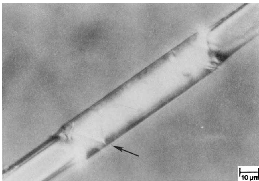
Fig. 11. Transmission optical micrograph of fibers spun at 2500 m/min and at a quench-air temperature of 40°C elongated 3% at 20%/min strain rate showing shear bands (arrow) prior to neck formation.
